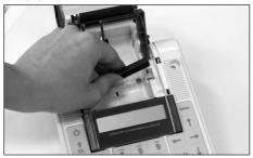
4 Hold the ends of the ribbons upended through the display and return the printer roller (3) to the
