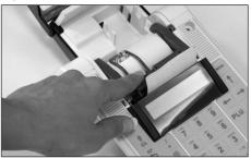
5. Press the paper-feed button (4) to be sure the roll properly advances.
