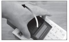
2. Press the printer roller release lever to release the printer roller, and then lift it.
